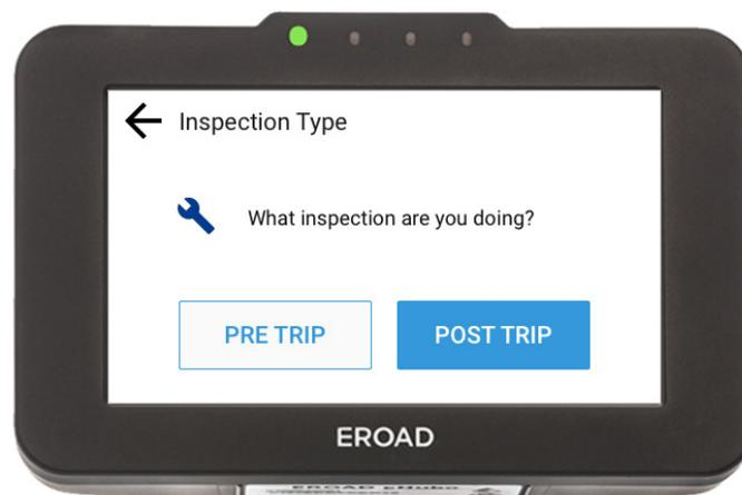
*Intuitive in-vehicle touchscreen allows drivers to report as well as certify vehicle defects are repaired*
